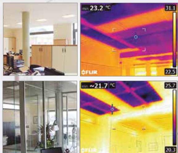
Heating and cooling process example.
